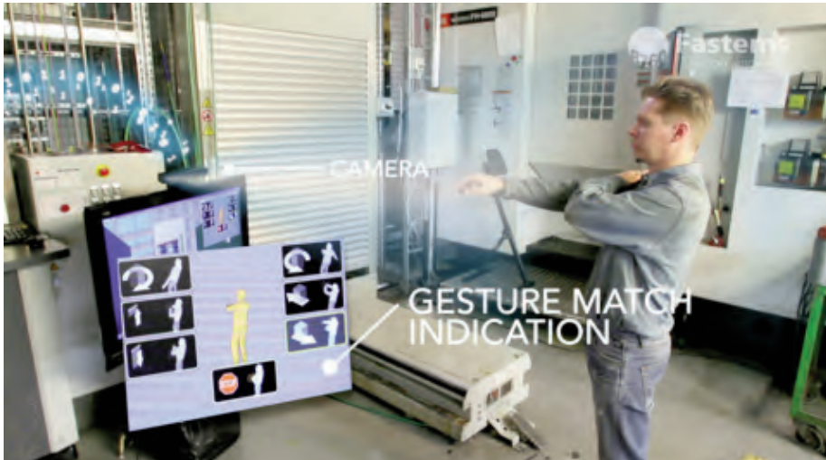
Figure 1. The prototype created within UXUS for demonstrating gesture control of loading stations
